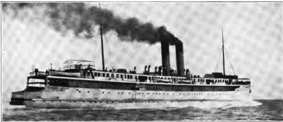
Fig. 37. — Sea-going Train Ferry Steamer Dröttning Victoria .
